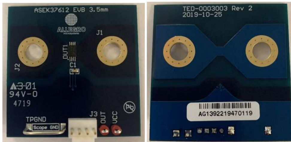
Figure 26: PCB Top (left) and Bottom Layers (right), 3.5 mm copper width below sensor
