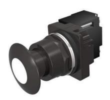
30mm BlackMax, Epoxy Coated Corrosion Resistant Complete Metal Unit Illuminated Push-Pull Operator Full Voltage, 24V AC/DC Incandescent Lamp Mushroom Head Cap Small 1 3/4" (44.5 mm) Metal, Black with White Lens 3 Position Pull-Momentary/Push-Maintained UL Listed, CSA Certified NEMA 1,3,3R,4,4X,12,13 & Automotive Standards
