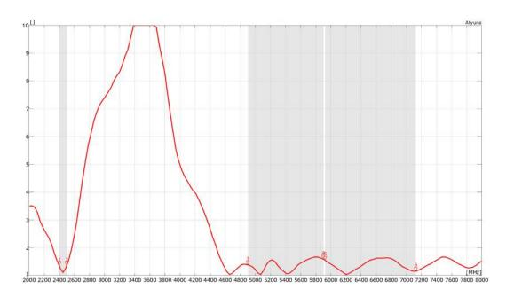
All data measured on SRF3W077 in a loaded condition adhered to a 2mm thick ABS carrier
