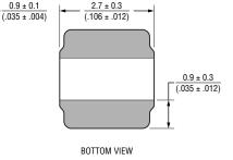
Note: Top and side view dimensions do not include termination. For maximum overall dimensions including termination, add 0.1 mm.
