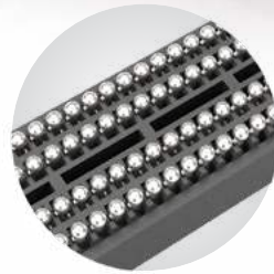
Solder ball technology for simplified processing
