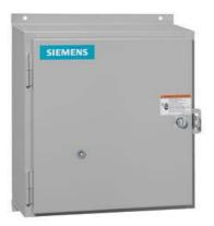
Non-reversing contactor, Size 1P, Single phase full voltage, Contactor amp rating 35A, 3 wire (NO aux included), 110-120/220-240VAC 60Hz coil, Non-combination type, Encl. NEMA type 4X fiberglass, Water/dust tight noncorrosive, Standard width enclosure
