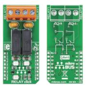
RELAY click<sup>™</sup> is an add-on board in **mikroBUS<sup>™</sup>** form factor. It's a compact and easy solution for adding RELAY to your design. It features two **G6D1AASI-5DC** power PCB relay modules as well as two screw terminals. RELAY click<sup>™</sup> communicates with target board microcontroller via **mikroBUS<sup>™</sup>** PWM (RL1) and CS (RL2) pins. The board is designed to use 5V power supply only. LED diode (Green) indicates the presence of power supply.
