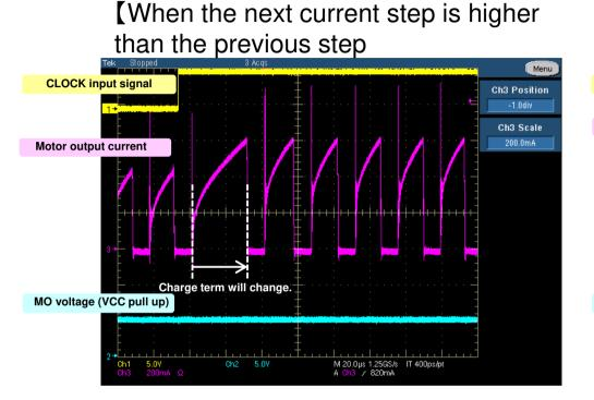
When the current threshold (current step) is shifted to the next threshold (step), the 'Charge' time may change, but the 'Decay (=off time)' time will not. (The off time depends on the OSCM resistance.) When the next current step is lower than the previous step
