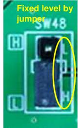
Jumper indicated in the left figure is adopted on this evaluation board to set operation of the TB67S149FTG. To select the function by the jumper, short-circuit JPCC. Fixed level of the silk near the jumper is indicated inside the white frame. Please change the short position according to the configuration of the usage function.
