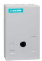
Non-reversing NEMA contactor, Size 1, 4 power poles, Contactor amp rating 27A, 3 wire (NO aux included), 110-120/220-240VAC 60Hz coil, Non-combination type, Enclosure NEMA type 1, Indoor general purpose use, Standard width enclosure
