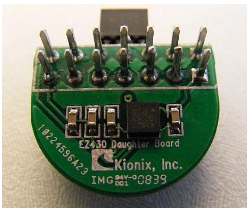
Figure 4: Kionix EZ430-7 Evaluation Board Mounted on TI eZ430-T2012
