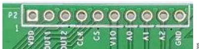
Figure 5. Connector P2 for Access to the SPI of the ADC of the EVAL-ADA4570SDZ
