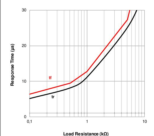
Testcondition:  $I_F = 5mA$ ;  $TA = 25^{\circ}C$ Testcondition:  $I_C = 2mA$ ;  $V_{CF} = 2V$ ;  $TA = 25^{\circ}C$
