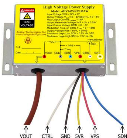
Figure 2. The Connecting Lead Wires of AHV24V4KV1MA
