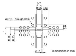
Line width be designed to match  $50\Omega$  characteristic impedance depending on PCB material and thickness.
