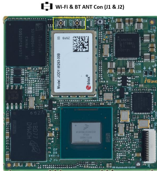
Figure 3: Wi-Fi and Bluetooth Antenna Connector
