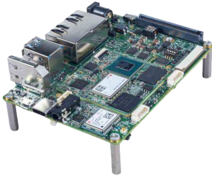
Figure 6: i.MX 8M Plus OSM Development Platform
