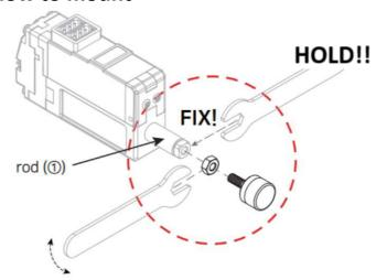
Pay attention not to apply excessive turning force to the rod (1) when installing the end tip to the rodend. Otherwise, it may cause product damage.
