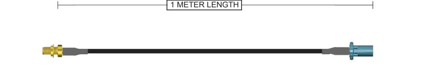
Connector A 132119 SMA Jack Straight Bulkhead - Rear Mount Brass Gold + Heatshrink 50 Ohm RG-174 Continuity/Hi-Pot Connector B 2FA1-NZSP-C01Y1 FAKRA Plug Straight Zinc Nickel + Heatshrink
