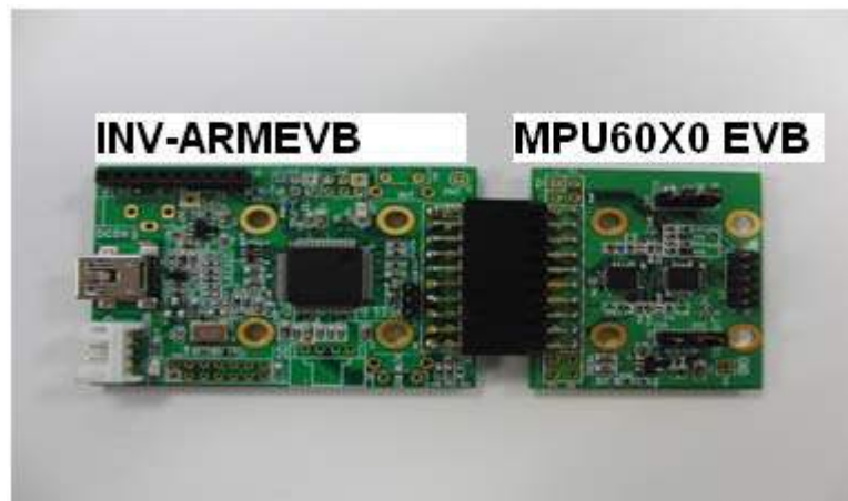
Figure 4. MPU-60X0 EVB connected to ARM Board
