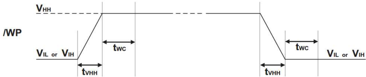
Figure 66. ACC Program Acceleration Timing and Voltage Levels
