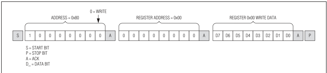
Figure 28. Format for I 2 C Write
