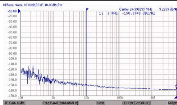
Figure 49. Output 1/2 = 156.25MHz LVPECL RMS Jitter is 520 fsec (10 kHz to 20 MHz)
