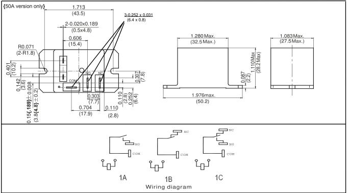
Dimensions in inches with metric equivalents in parentheses. Tolerance: ± .010"
