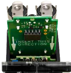
Figure 1. Q45 battery board
