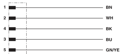
Contact assignment of the M12 plug
