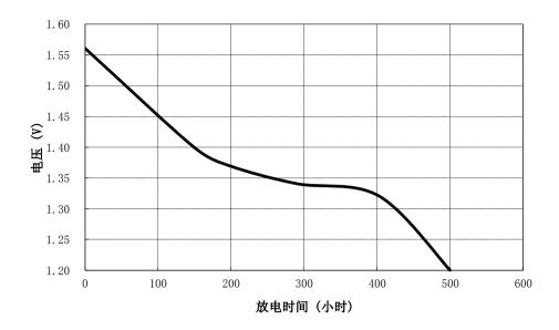
Discharge method:  $68k\Omega$ , 24hours/day, E.V. 1.2V Temperature:  $20\pm2^{\circ}$ C
