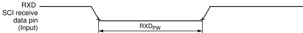
Figure 10-15 RXD Pulse Width
