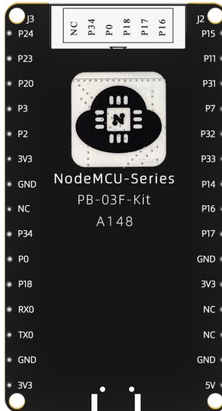
Figure 7 Schematic diagram of development board pins (bottom view)
