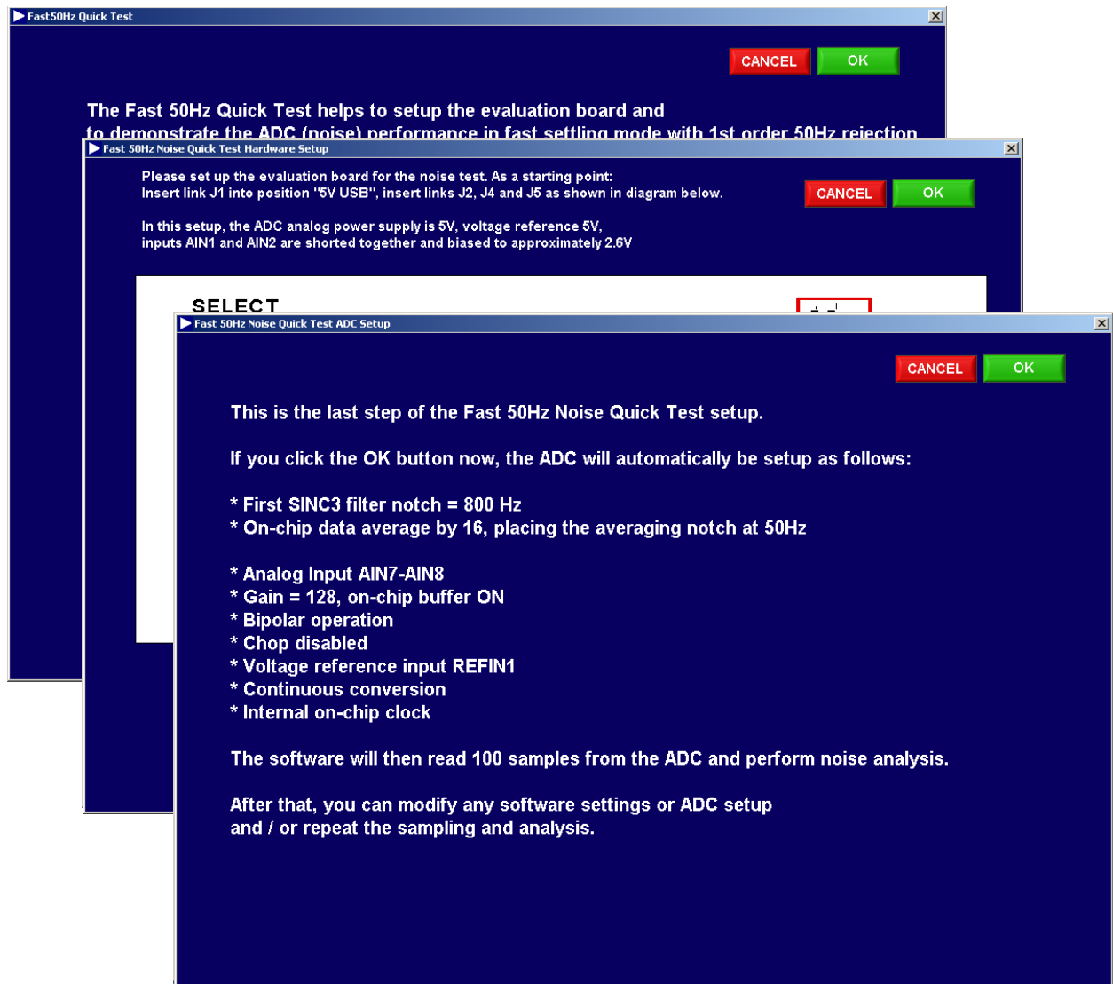
Figure 9. Fast 50 Hz Quick Test
