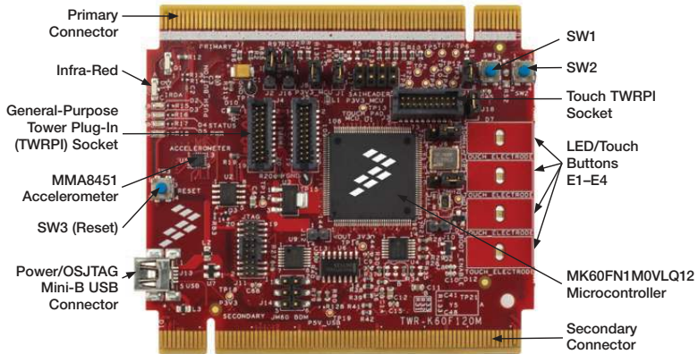
Figure 1: Front side of TWR-K60F120M board (TWRPI devices not shown)
