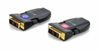
The TL-FO-DVI is a mini DVI optical fiber extender, including a transmitter and a receiver. It is compatible with HDMI video up to 4Kx2K/30Hz, and extends HDMI/DVI video up to 300m via single optical fiber cable with EDID management.
