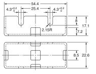
Note: The Cover has five holes for easy lead wire connections.
