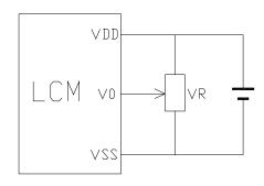
V<sub>DD~</sub>V<sub>0</sub>: LCD Driving voltage
