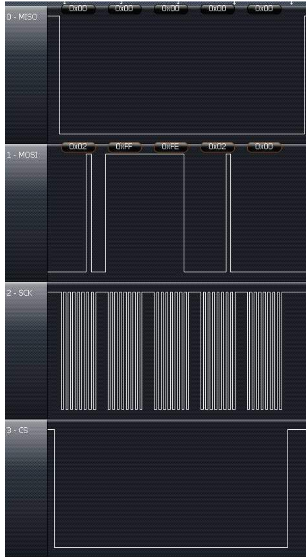
Figure 5-8. SPI Access Example: Write of the Control Register at Address 0xFFFE With 0x00, 0x02 (RF Enable = 1)
