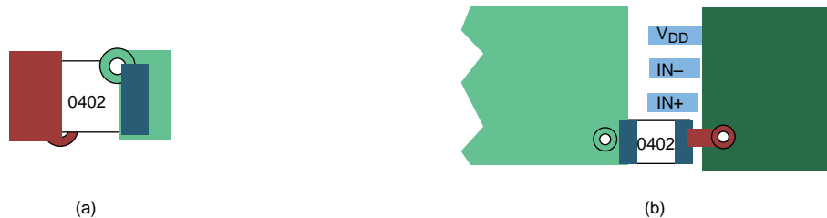
Figure 29. Typical Decoupling Capacitor Layouts
