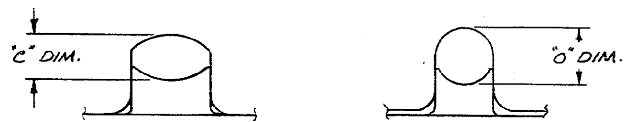
BARREL CRIMP INSULATION CRIMP ENLARGED VIEW OF CRIMPS
