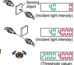
③ Turn the threshold value adjuster to the threshold value [in the digital display (green)] that is the value in between ① and ②. (The threshold value is automatically written to the EEPROM.)
