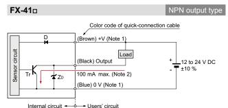
Notes: 1) The quick-connection sub cable does not have +V (brown) and 0 V (blue). The power is supplied from the connector of the main cable.
