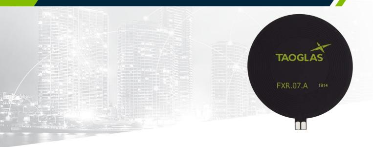
The FXR.07.A is a circular, flexible, NFC (Near Field Communications) antenna for use in mobile devices and other applications. The design provides a flexible NFC antenna that can be adhered to the plastic enclosure of the device for ease of installation.
