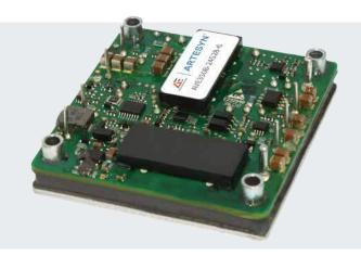
Advanced Energy's Artesyn AVE350B series of isolated DC-DC converters is designed specifically to provide the main 28 Vdc supply for RF power amplifiers in small-cell, low power and remote radio head (RRH) telecommunications applications. The series comprises two single output models: the AVE350B-24S28-6, which accepts a wide range input of 18 to 36 Vdc; and the AVE350B-48S28-6, which accepts a wide range input of 36 to 75 Vdc.
