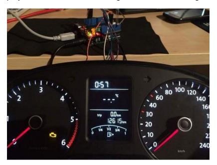
Ever wanted to play a car/truck simulator with a real dashboard on your PC? Me too! I'm trying to control a VW Polo 6R dashboard via CAN Bus with an Arduino Uno and a Seeed CAN Bus Shield. Inspired by Silas Parker. Thanks Sepp and Is0-Mick for their great support!
