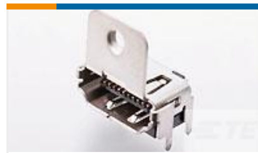
TE Part #1-1747981-4 Std HDMI, RA, SMT, Panel grd, Flange
