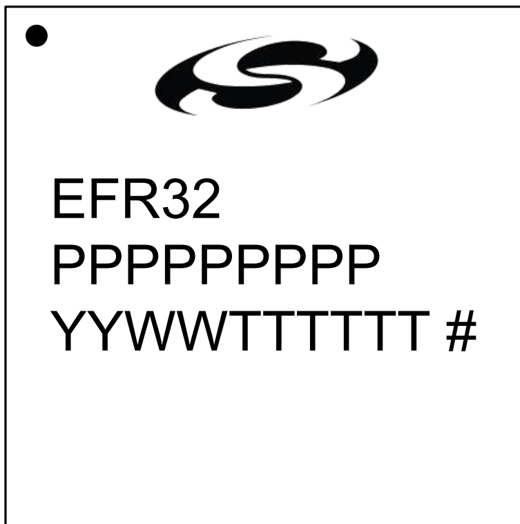
Figure 7.3. QFN48 Package Marking
