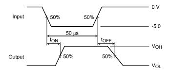
Note 1: Pulse width 50  $\mu s$ , Duty cycle 10% Output impedance 50  $\Omega$ , tr  $\leq$  5 ns, tf  $\leq$  10 ns
