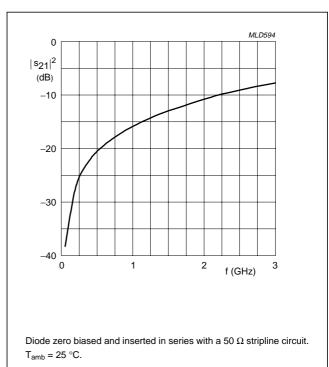
Fig.5 Isolation  $(|s_{21}|^2)$  of the diode as a function of frequency; typical values.
