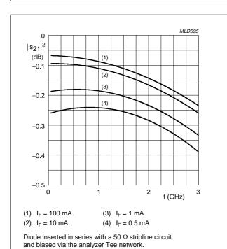
Fig.4 Insertion loss  $(|s_{21}|^2)$  of the diode as a function of frequency; typical values.
