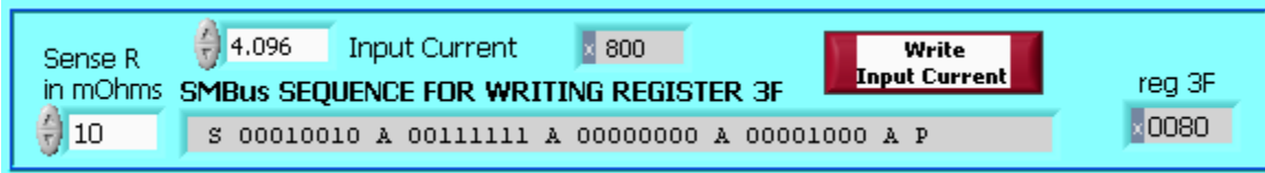
FIGURE 11. WRITE INPUT CURRENT BUTTON
