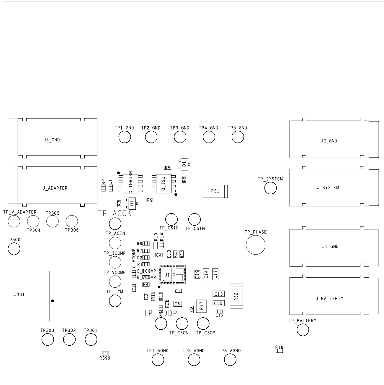
FIGURE 20. BOTTOM SILK SCREEN (VIEWED FROM THE BOTTOM)
