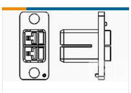
TE Part #292353-1 RECEPTACLE HOUSING FOR 2P HIGH CURRENT D
