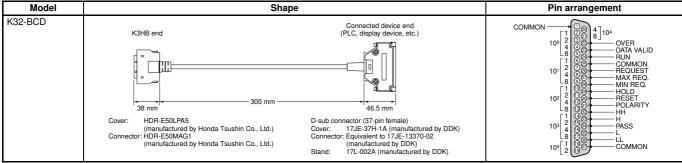
Note: The BCD Output Cable has a D-sub plug. Cover: 17JE-37H-1A (manufactured by DDK); Connector: equivalent to 17JE-23370-02 (D1) (manufactured by DDK)
