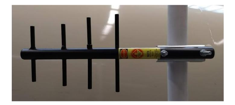
Antenna mounted vertically on post with insulator on driven element facing up
