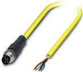
Sensor/Actuator cable, 4-position, PVC, Yellow RAL 1021, Plug straight M8, on Free cable end, Cable length: 5 m
