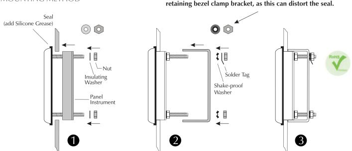
Notes: On some panel instruments it may be easier to configure links and calibrate the product prior to fitting the instrument and BEZ 700-IP into the panel. Always observe safety warnings on the Panel Instrument datasheet. Do not allow connections to touch the metal bezel, as this may adversely affect product safety or stop the panel instrument from functioning correctly.
