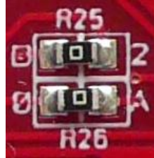
Figure 6 - GPIO Swap Resistors
